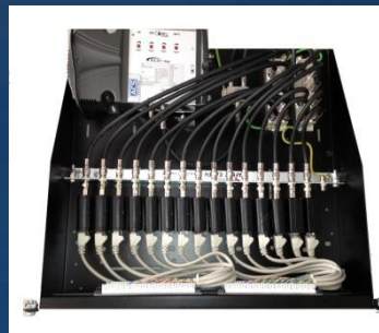
Customised product containing converters, amplifiers, patch leads, coax fly leads and distribution units.
